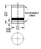
Plastic case MELF (DO-213AB) Dimensions in millimeters
