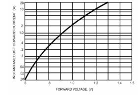
FIG.2- TYPICAL FORWARD CHARACTERISTICS
